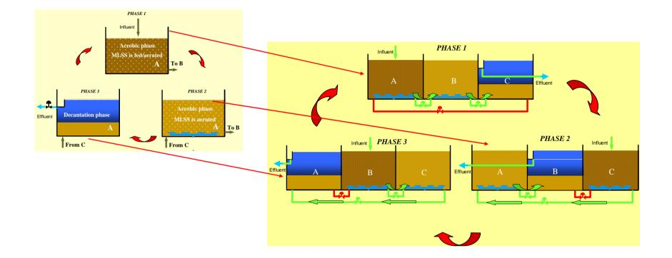
Seen over the <u>complete cycle</u> each <u>unit</u> has a SBRcyclic operation, however <u>without level changes</u> The LUCAS system combines the advantages and disregards the disadvantages of the conventional WWTP and the variable volume Sequencing Batch Reactor WWTP
