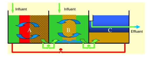
LUCAS-3 NPremoval **(high NP)** A: Anoxic / anaerobic/aerobic B : Anoxic/aerobic/anoxic
