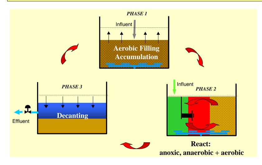
Time & alternation of 'react' phases is adapted to obtain optimal nutrient removal
