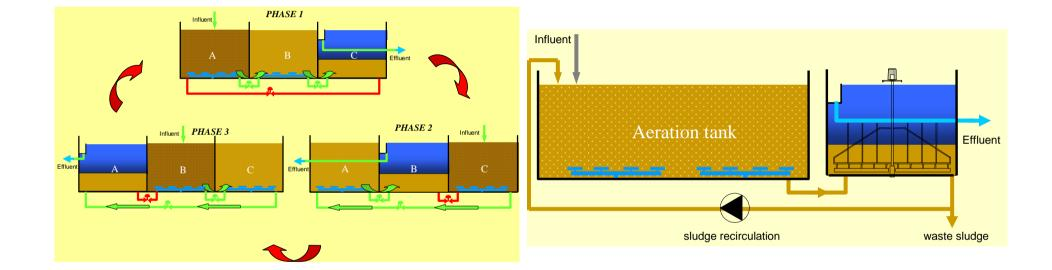
Seen over each <u>partial time phase</u> the <u>combination of the individual</u> <u>units</u> (the overall tank) resembles a continuous conventional activated sludge system, however <u>without the sludge recirculation</u>
