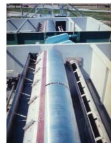
Our fixed VOC containment cover systems reduce the risk of explosions by using an inert gas, such as nitrogen, instead of air.
