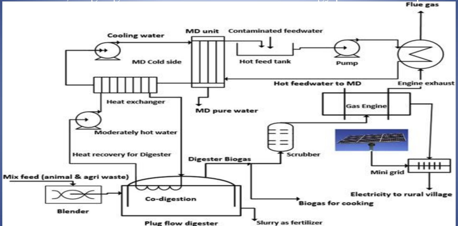
Excess digester gas is employed for cooking and lighting, while waste heat from the process derived a AGMD unit for desalination
