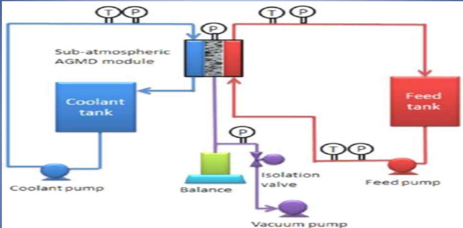
The Flux of V-AGMD module is measured to be 3 times the flux of single stage AGMD
