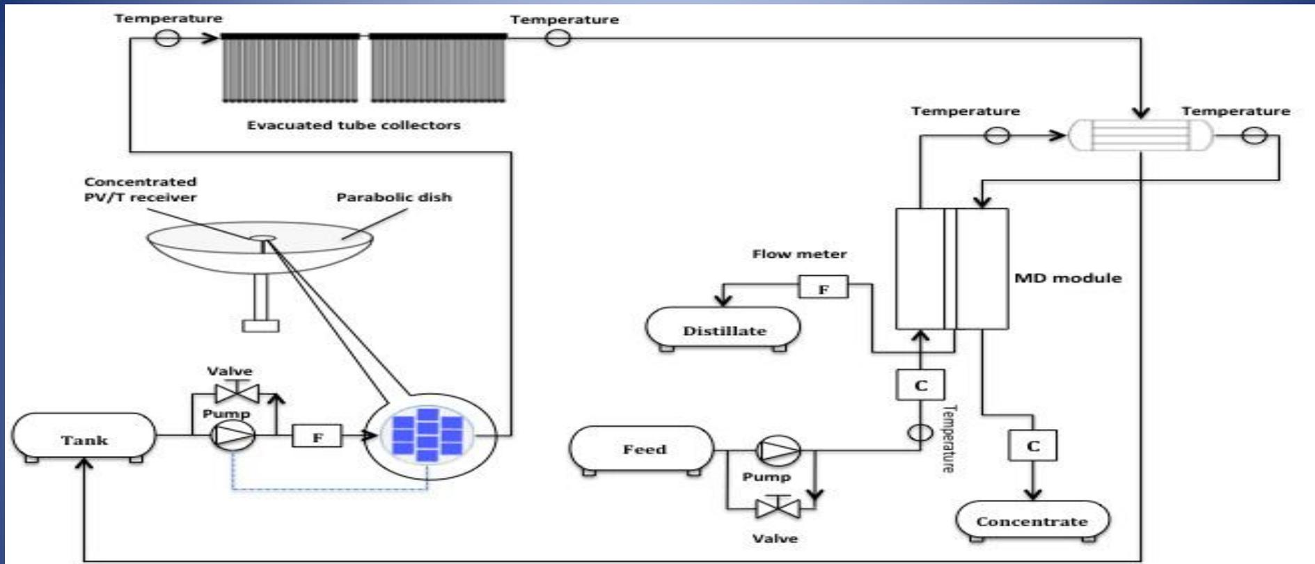
This integration provides two types of energy; (1) a thermal energy which is required to drive the AGMD unit, and (2) an electrical energy which is required to power the pump and tracking devices. Flux of  $3.4 \text{ Kg/m}^2\text{h}$  and a conductivity of  $35 \mu\text{s/cm}$
