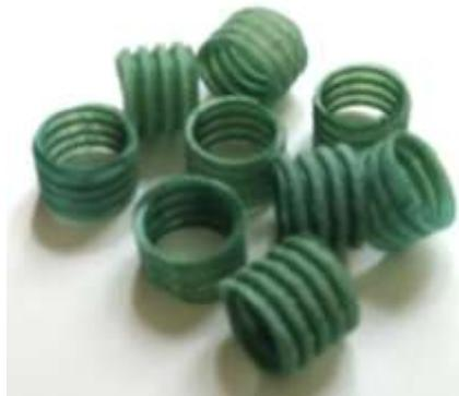
**Figure 2** Biofilm carriers used in experiments
